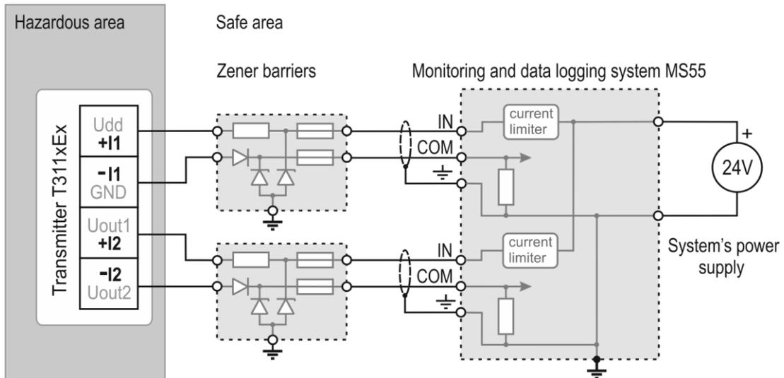
**Example of the T311xEx transmitter connection to the inputs of monitoring and data logging system MS6 (COMET) using Zener barriers type MM 7087+ (MM GROUP).**
