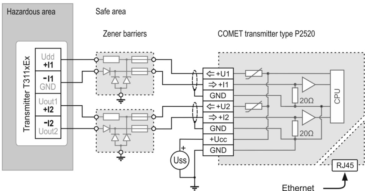
**Example of the T311xEx transmitter connection to the inputs of monitoring and data logging system MS55 (COMET) using Zener barriers type MM 7087+ (MM GROUP)**
